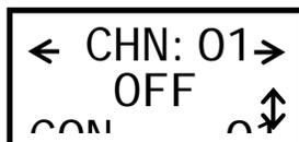
Use the ← and → buttons to cycle through the channels (1 - 24) and use the ↑ and ↓ buttons to turn the channel ON or OFF for the step.
