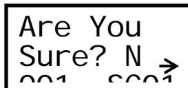
The N means NO. Use the → button to change it to Y (yes) and push ENTER. The function will proceed.
