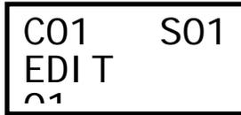
The chase which is to be programmed is shown in the upper left (C01 meaning chase 01). The step number within the chase is shown in the upper right (S01 meaning step 01). The item on the bottom row (EDIT) will access a submenu enabling you to edit that chase/step number.
