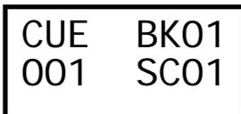
The left side of the display shows the cue number being assigned. The upper right shows the bank number of the scene assigned to that cue. The lower right shows the scene number (within the bank) assigned to that cue.
