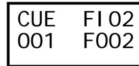
The cue number is shown on the left side of the display. The right side shows the fade in time in seconds on the top and the fade out time in seconds on the bottom.
