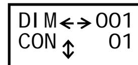
The top row shows a dimmer channel number. The bottom row shows the console channel (fader) to which the dimmer channel number is assigned. Use the → and ← buttons to cycle through the dimmer channel numbers. The assigned console channel will be shown for each one. You can change the console channel number with the ↑ and ↓ buttons.
